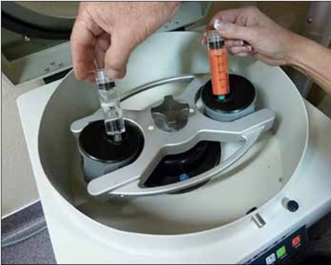
Figure 7a. AdiPrep centrifuge. 4 minute cycle at approximately 1000 g force, showing tissue processing syringe (with disk) on right. Harvest Technologies, Plymouth, MA.
